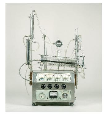
DATE: 1956. To bypass the cardiopulmonary circulation catheters are placed in the inferior and superior venae cava. These direct venous blood to a venous reservoir, heat exchanger, oxygenator and roller pump. The roller pump propels arterialized blood through the filter and bubble trap. The blood then is returned to the patient through a catheter in the femoral artery.
