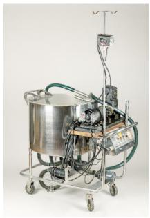
DATE: 1969; Parts: tubing, arterial and venous pressure monitors, blood pump, heparin pump, dialyzer inflow pressure monitor, dialyzer, air trap & detector, air tubing clamps. Use- to remove unwanted waste products from blood and balance electrolytes and minerals
